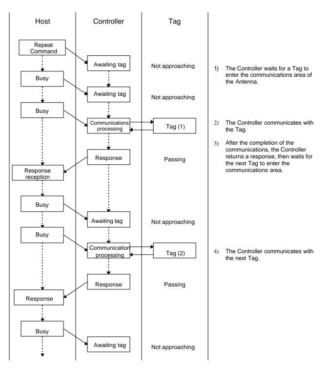
To send another command from Repeat Mode, be sure to use either the stop command or reset command, and make sure that the Controller has finished processing commands and is in command waiting status before sending the new command.
