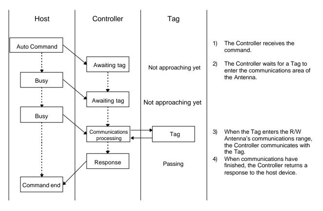
In Auto Mode, the communications path between the host device and the Controller is busy until a Tag approaches the Controller, so the host device cannot send the next command.
