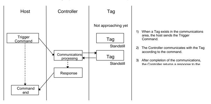
**Note**: Before using Trigger Mode, check that the Tags are not moving and are within the Antenna's communications range.
